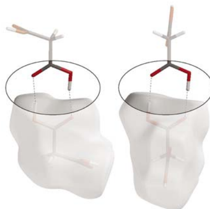
Figure 32 The different cyclic hydrogen bonds at the two ends of a malonic acid molecule in the crystal, highlighting the different ring arrangements, and the resultant different shapes of the Hirshfeld surfaces.
